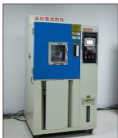
恒温恒湿 Constant temperature and humidity test chamber machine
